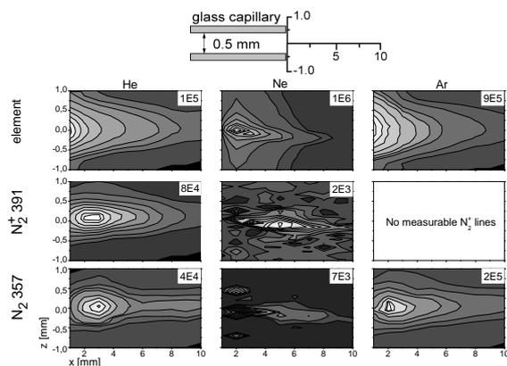
Fig. 2: Spatial density distributions of He,  $N_2^+$  and  $N_2$  measured in a He plasma jet compared with a Ne plasma jet and an Ar plasma jet, respectively. The maximum intensity is shown in the top right corner.
