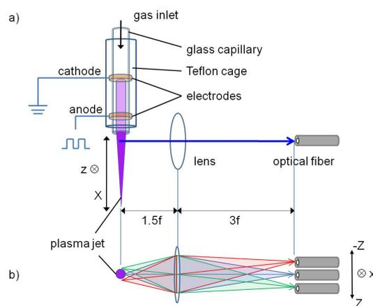
Fig. 1: Experimental arrangement for spatially resolved measurements a) top view, b) frontal view.
